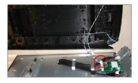
10.3 Disconnect the two screws fastening top USB bracket to the case and the two screws fastening PCB to bracket
